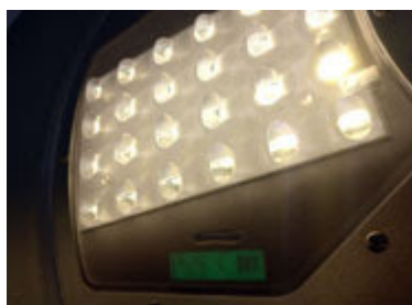
Battery power display.
