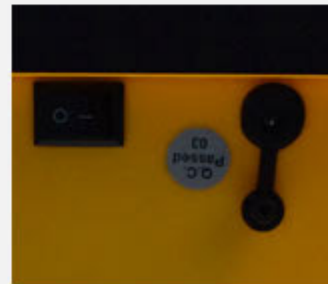
The bottom with switch and charging socket;
